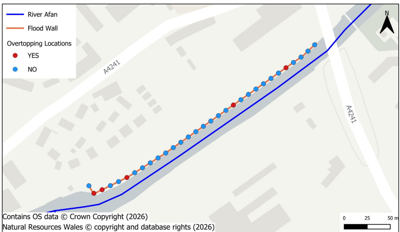
Figure 9: Overtopping Assessment Results
