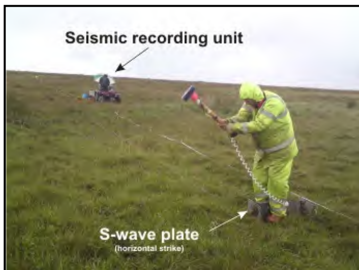
Plate 4: S-wave source plate (library picture)
