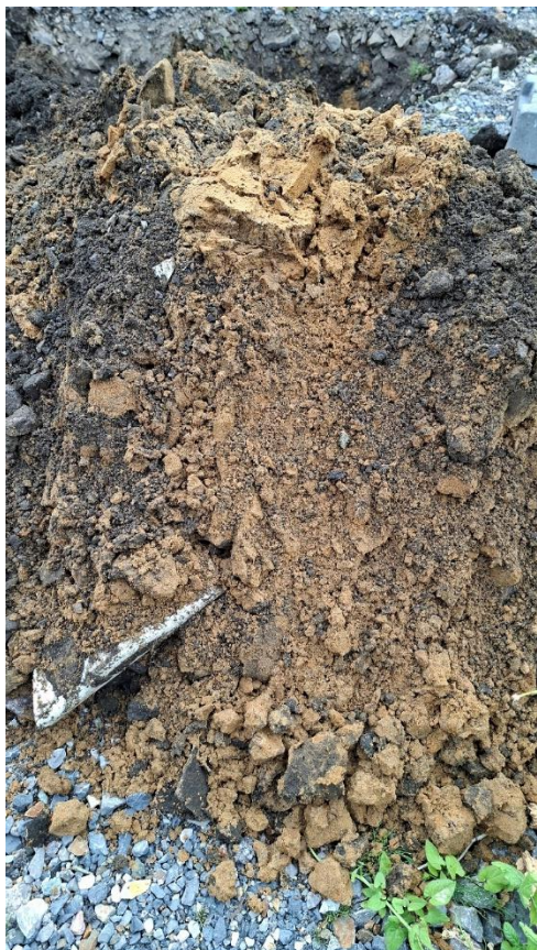
Figure 4 – Excavated soil, note high sand content
