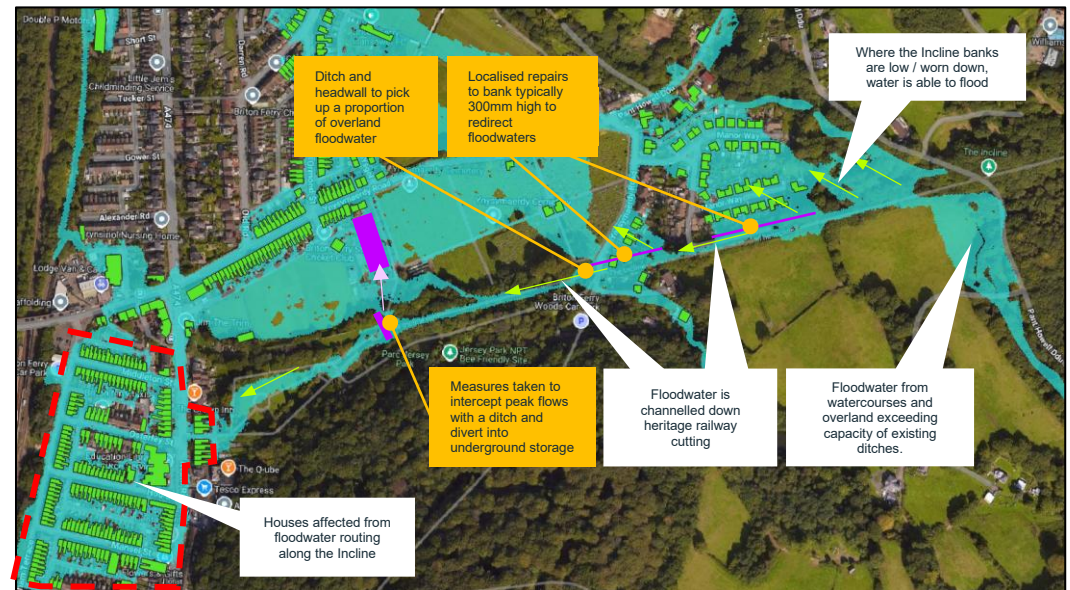
Figure 1-3 – Without scheme flooding extents near Jersey Park
