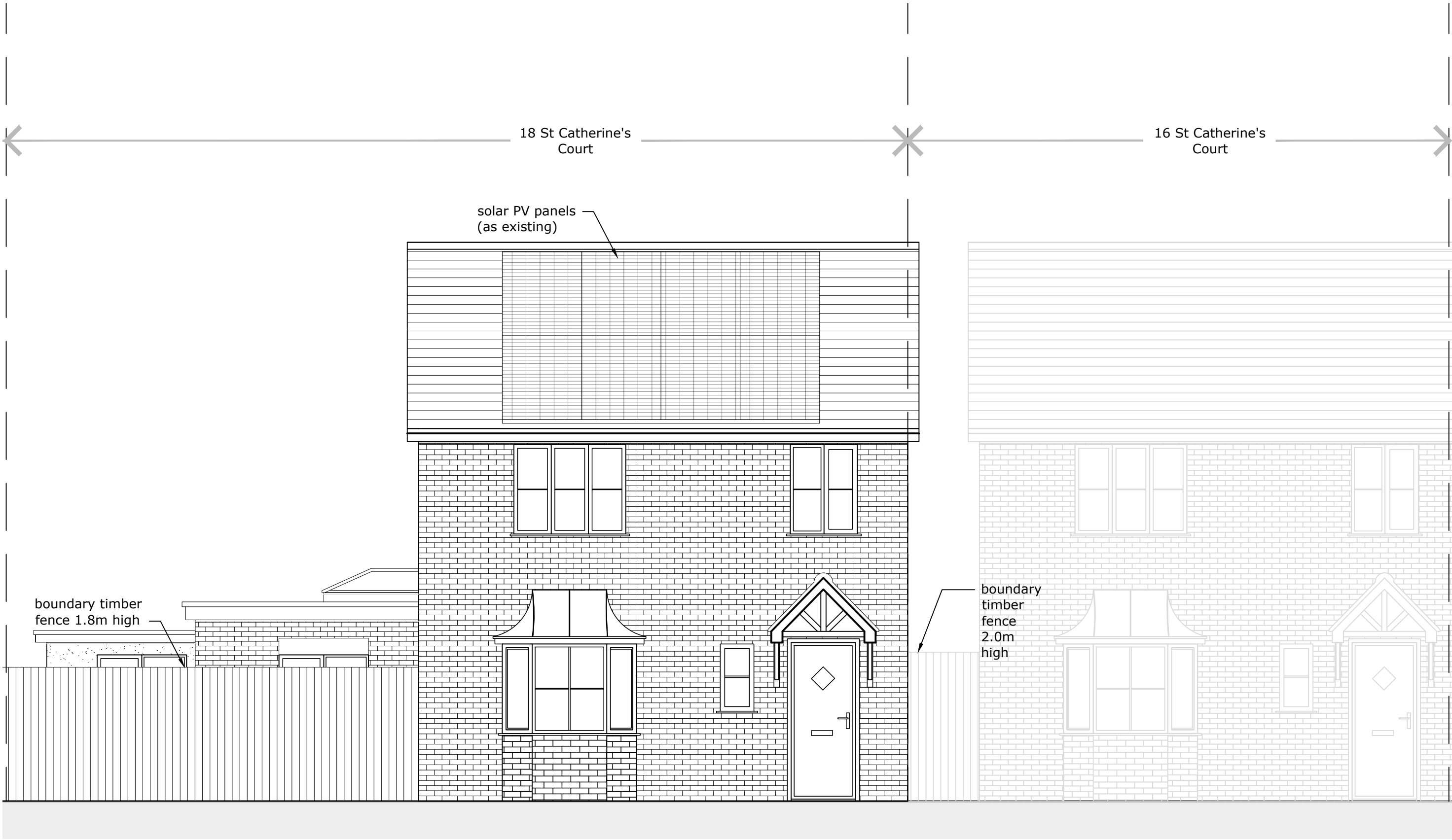
front elevation (south facing) as existing 1:50
