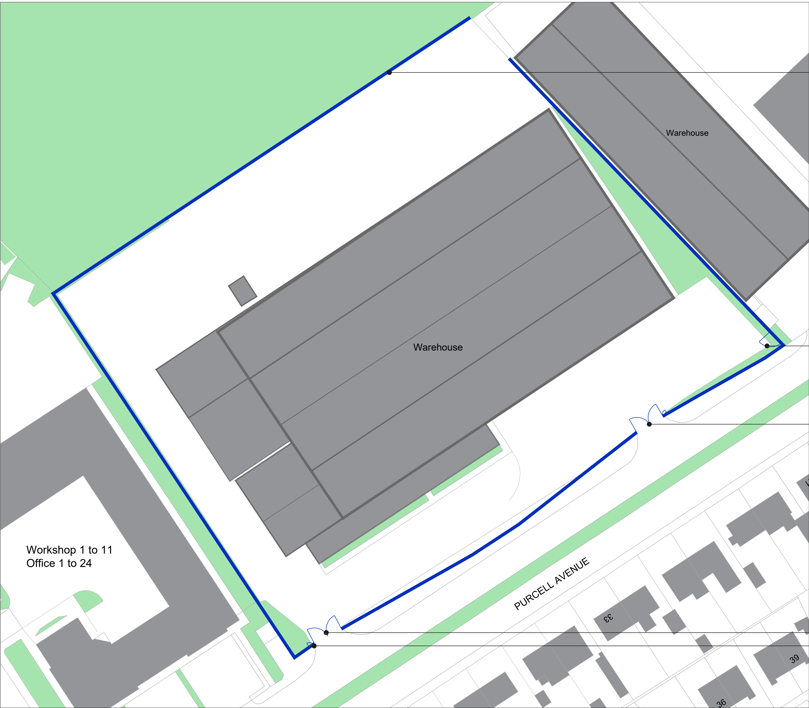
1 PROPOSED PLAN, SHOWING EXTENT OF NEW FENCE AND GATES Scale 1:500 @ A1
