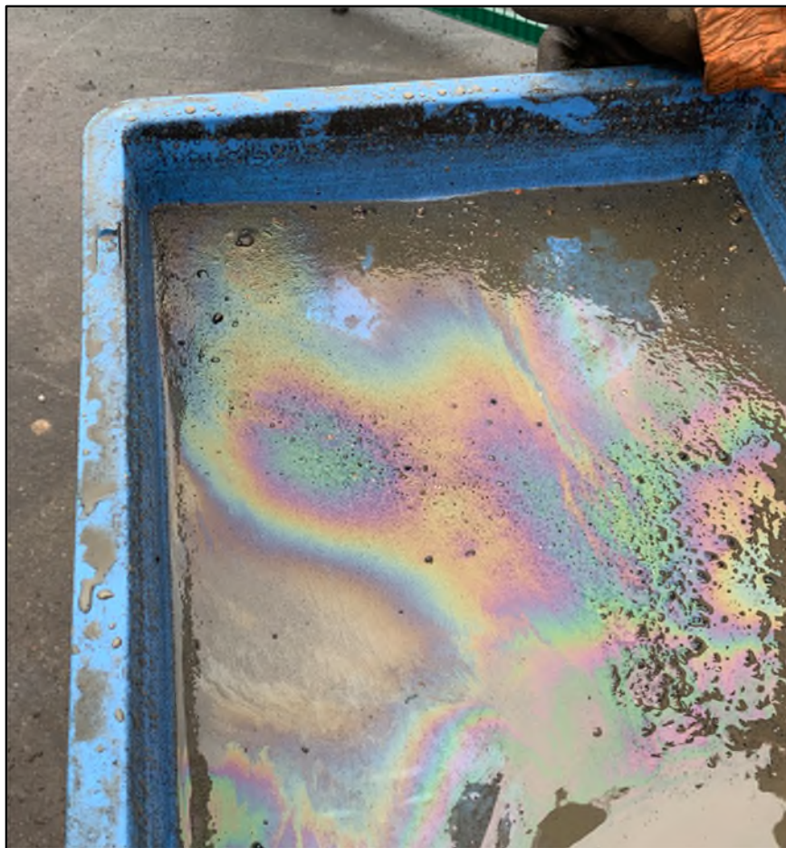
Figure 3.1 Groundwater collected from BH03 during drilling showing thin-film interference due to the presence of hydrocarbons.
