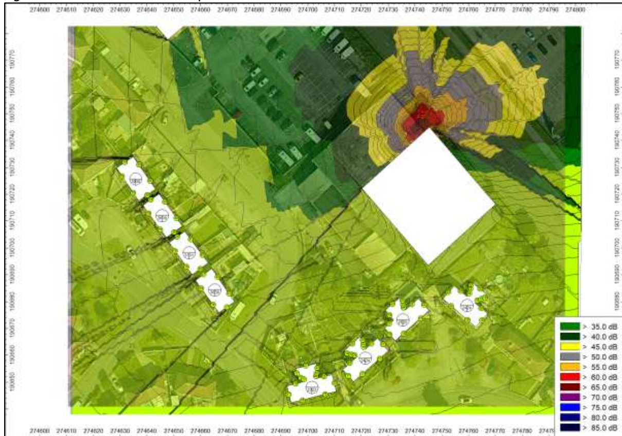
Figure 6: Predicted cumulative specific sound level
