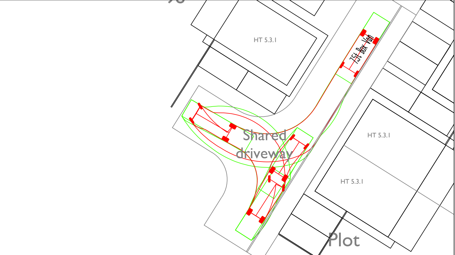
FIRE TRACKING AT PLOT 99
