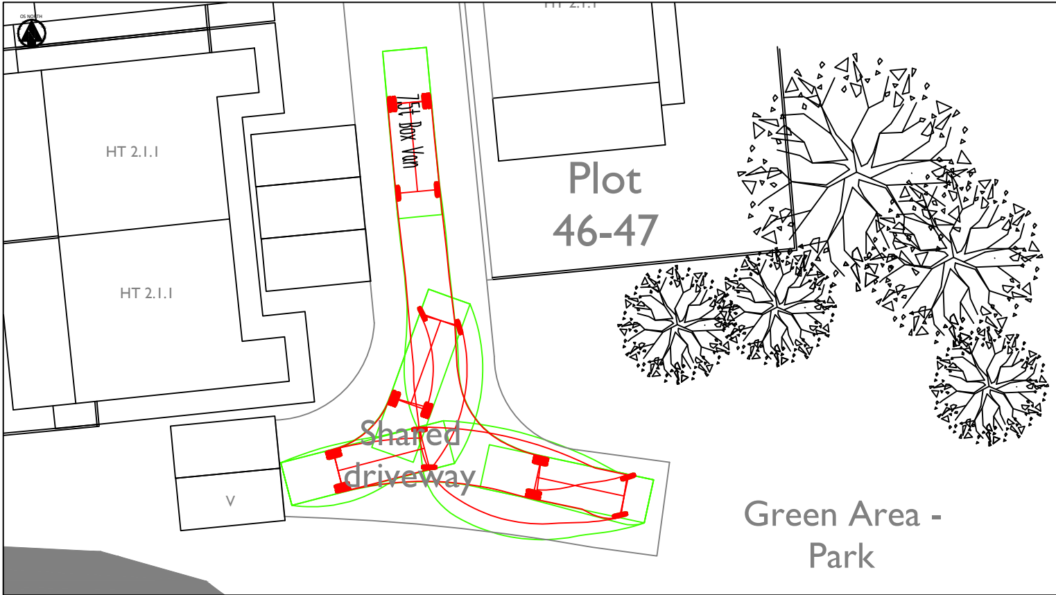
FIRE TRACKING AT PLOT 45
