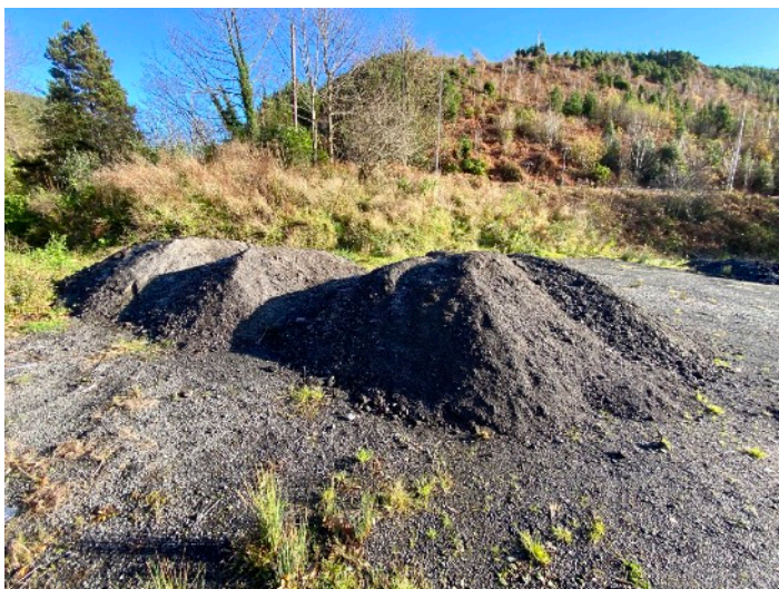
Stock piled crushed tarmac hardstanding in north east corner of northern car park
