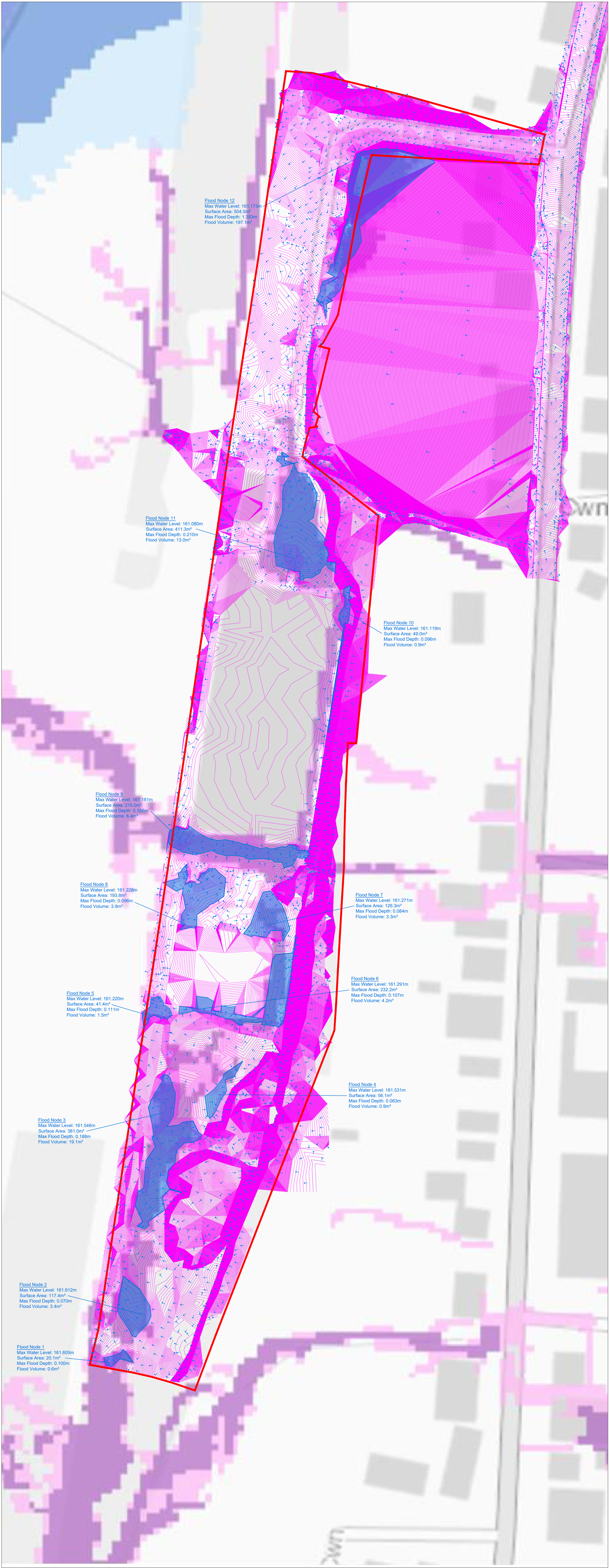
Analysis of existing on-site low-lying/surface water ponding areas and flood volumes based on site topographical survey Scale 1:500
