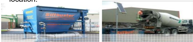
Fig.3.9 – Siltbuster settlement tank
