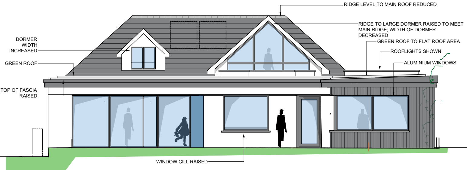
Rear (South Facing) Elevation 1:100
