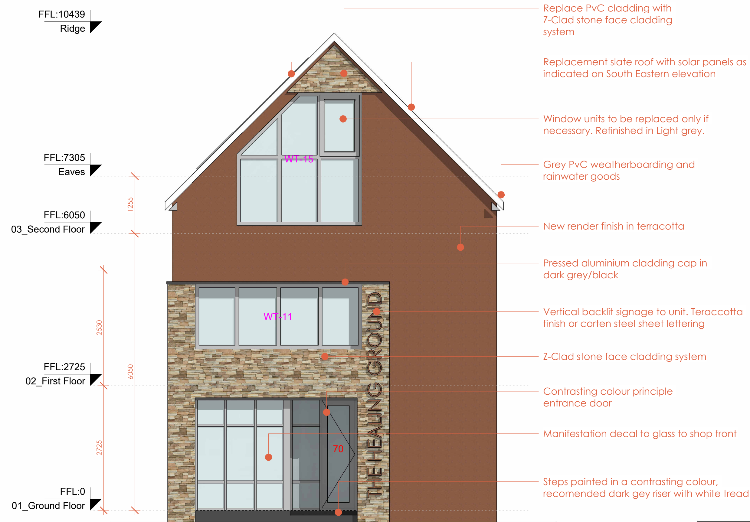
View No. 01 North Eastern elevation - Front 1 : 50
