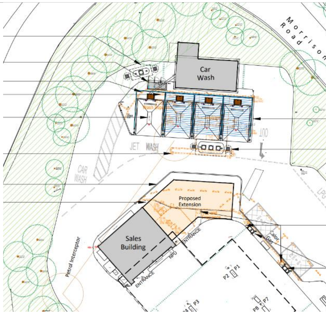
Image above: covering the valeting and extension works on the main petrol filling station.
