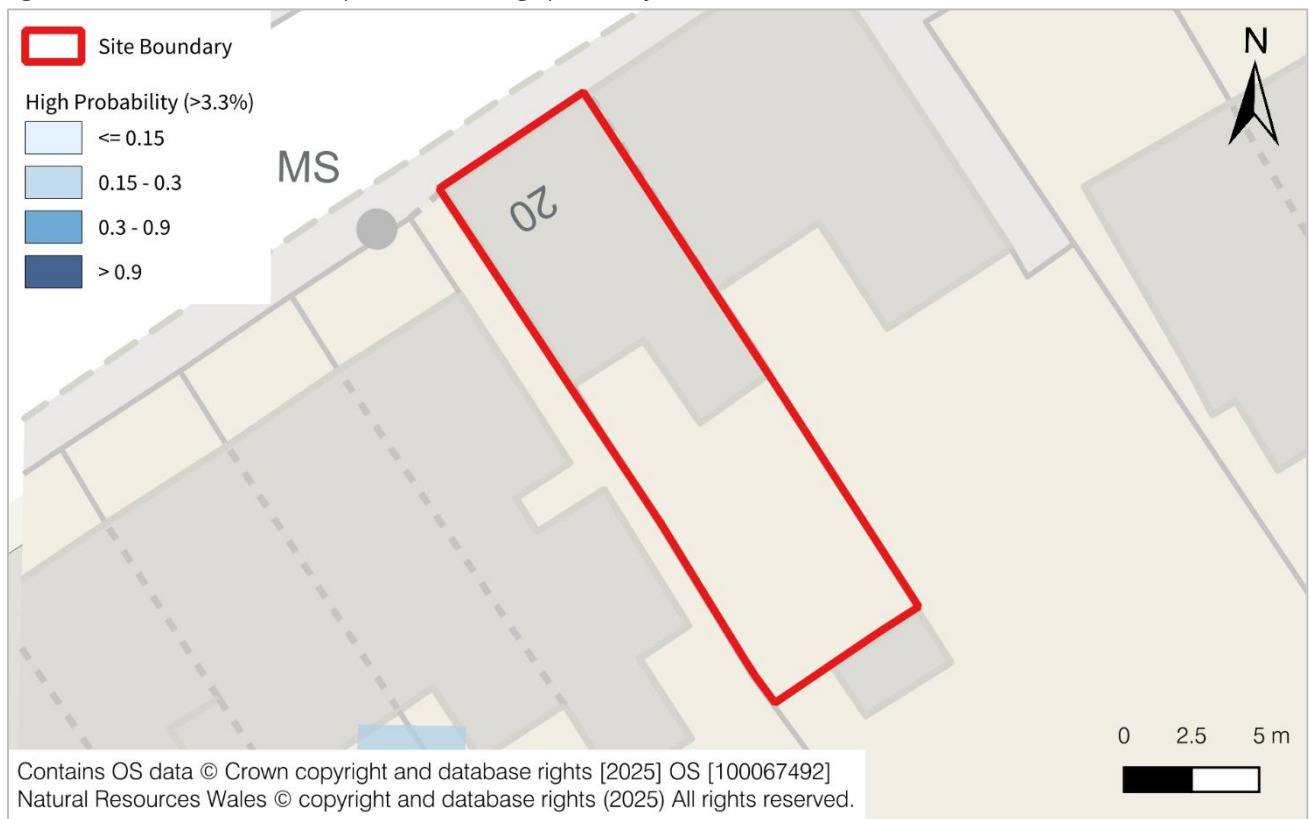
Figure 13 - Surface Water flood depths in meters (high probability)
