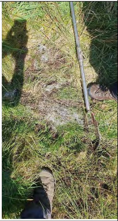
PSP09 – Borehole reinstated
