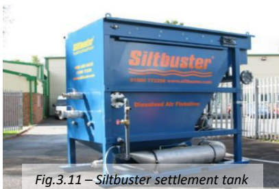
Fig.3.11 – Siltbuster settlement tank
