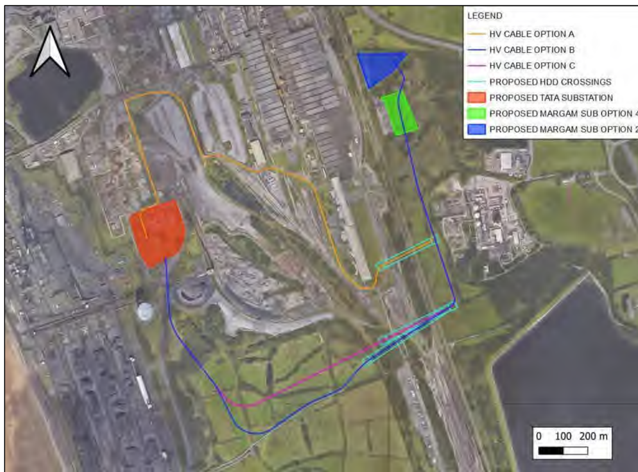
Figure 1.1. Site Plan showing proposed substation locations and cable route options.
