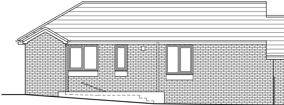
Existing Rear Elevation
