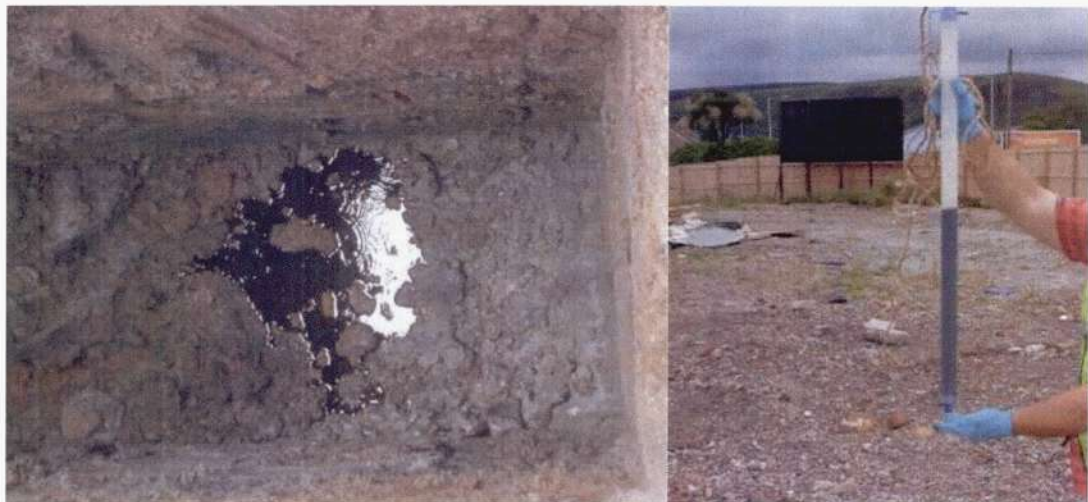
Figure 6A and 6B. Free phase gasoline type impacts in LEE Pit LP7 and recovered from Borehole E4 respectively.
