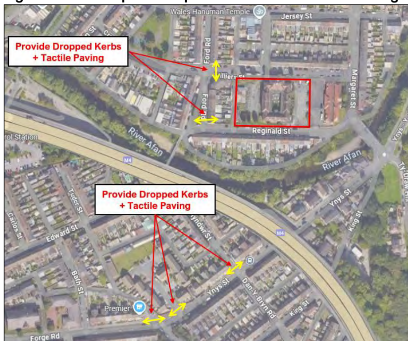
Figure 4B Proposed Improvements to Off-Site Walking Infrastructure
