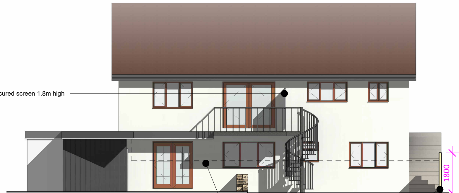
3 Proposed Rear Elevation (2) 1 : 100 Obscured screen 1.8m high Proposed boundary wall to be grey composite and 1800mm in height Boundary wall omitted for clarity
