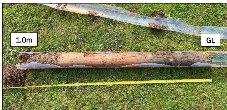
Insert 3 – View of windowless sample core recovery from GL to 1m in BH01. Note fine grained possible Alluvium beneath the Topsoil and above the coarse-grained River Terrace Deposits.
