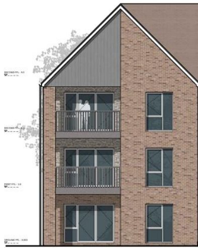
Figure 1: Existing Material Palette (Stone recess)
