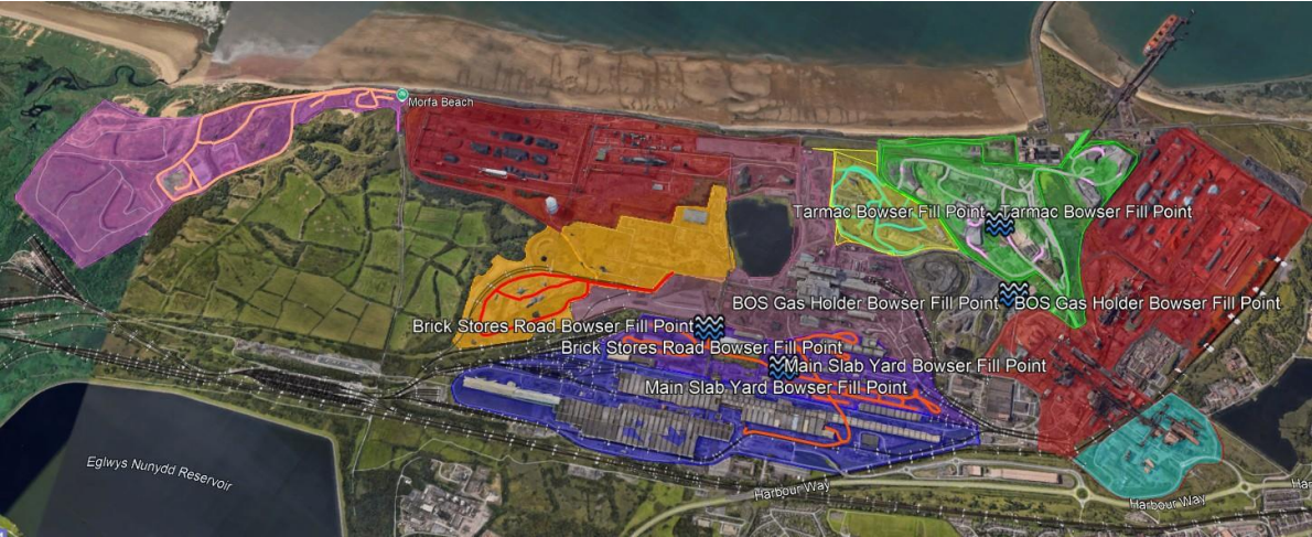
Figure 3.2: Location of onsite road dust suppression bowser systems
