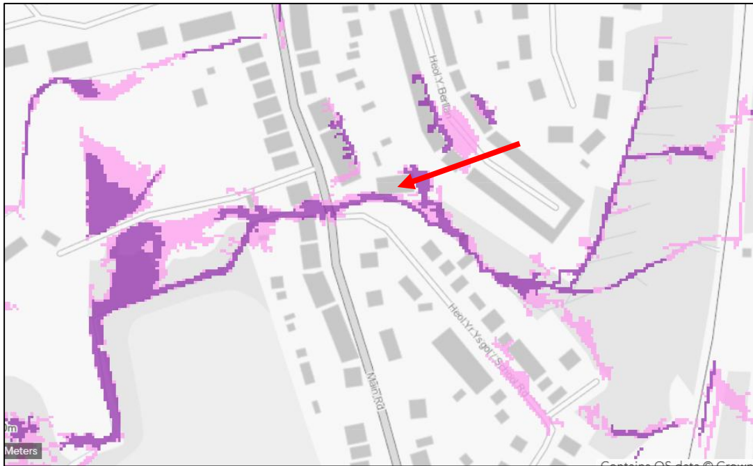
Figure 8 – extent of surface water flooding as extracted from Flood Map for Planning
