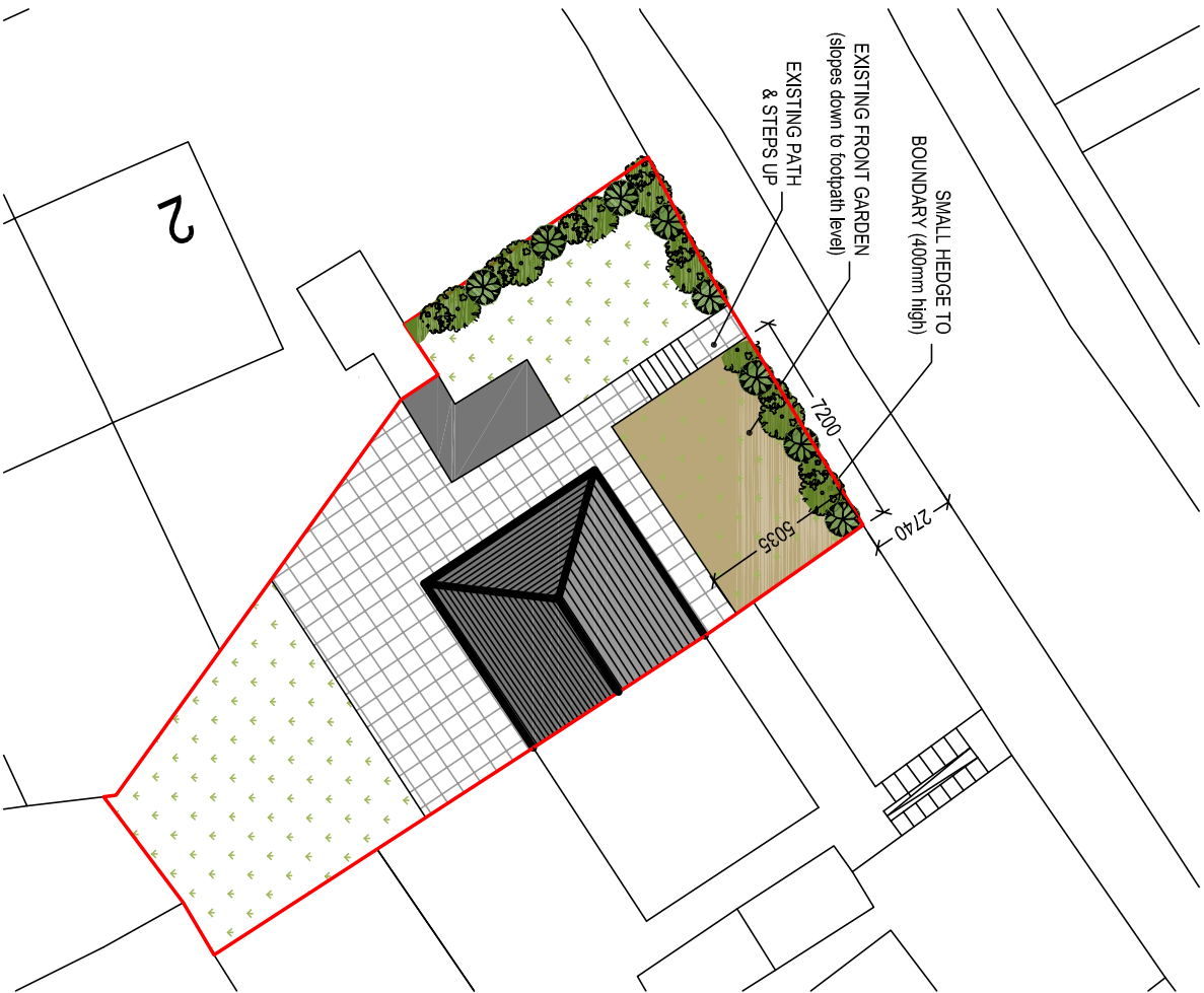
EXISTING SITE PLAN Scale 1:250
