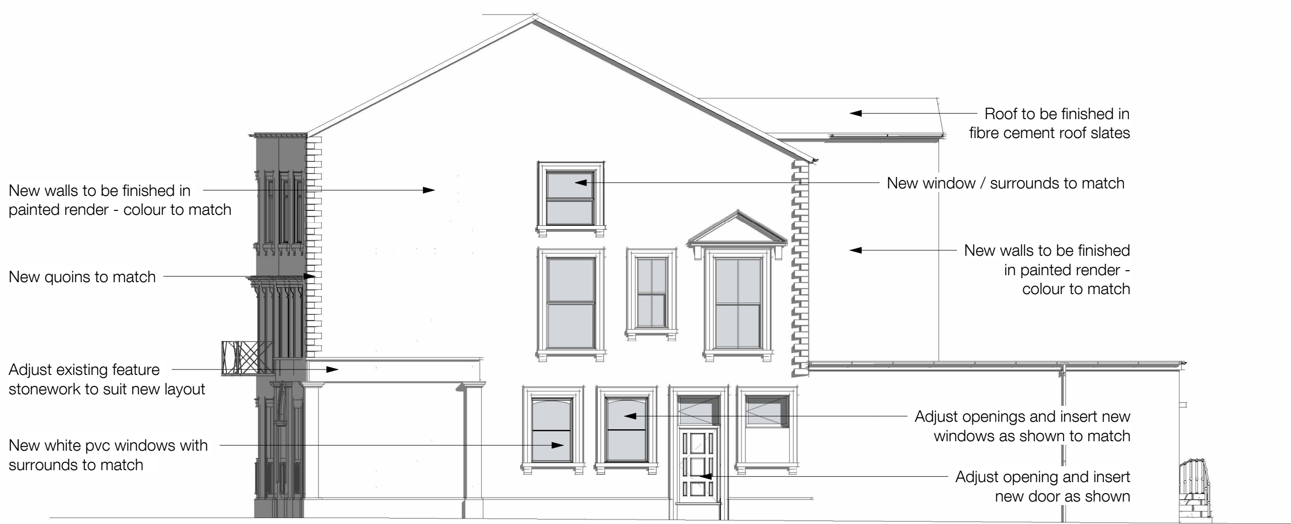
Proposed side elevation 1 : 100
