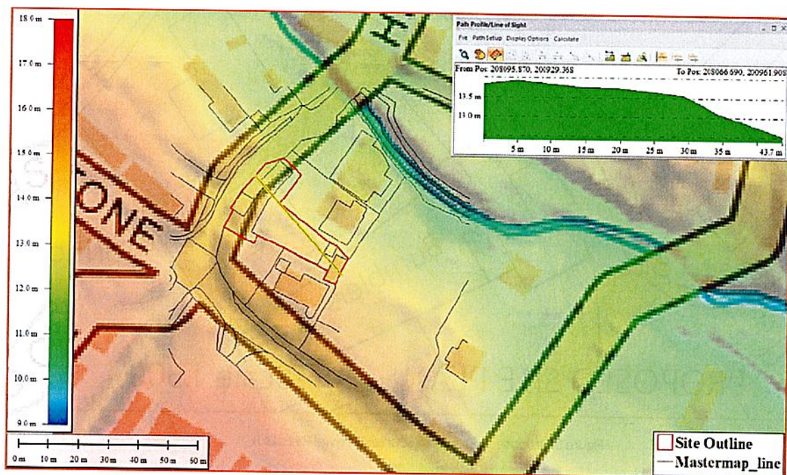
Figure 4: 2m LIDAR DTM showing topographic levels across the site. Transect runs from southeast to northwest. OS Mapping overlay. (Source: NRW, OS)
