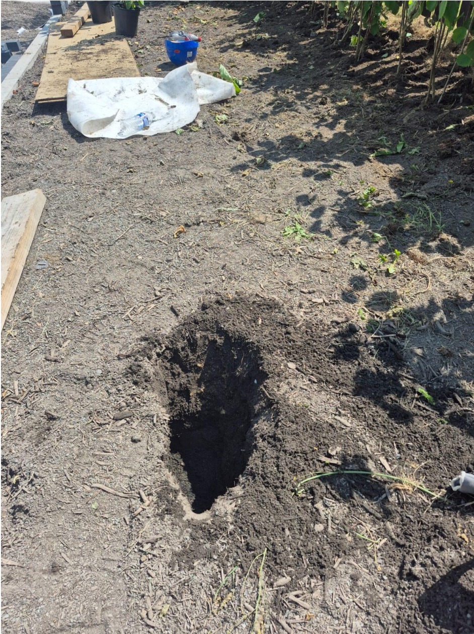
Plate 5: 450mm Thickness of Topsoil (Pit 3)
