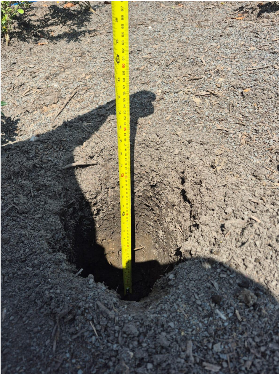
Plate 1: 450mm Thickness of Topsoil (Pit 1)
