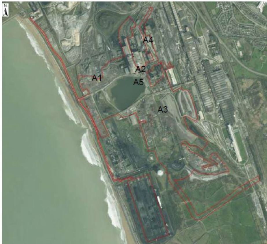
Figure 3-3 Five areas of different ground conditions
