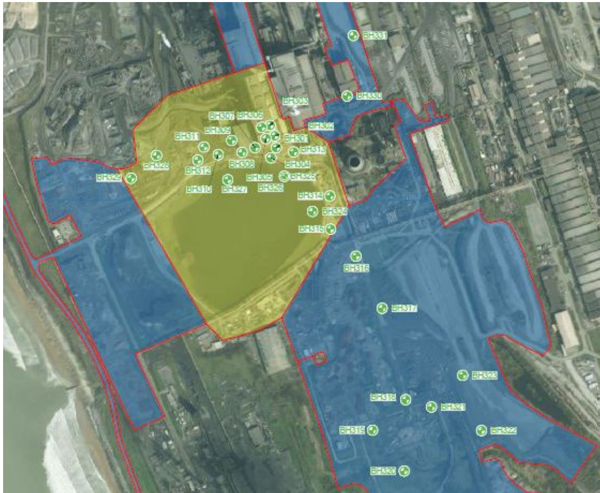
Figure 3-1 Site investigation Boreholes (yellow = Area 1, blue = Area 2)
