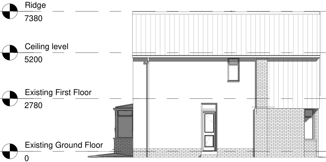
Existing Side Elevation (SW) 1 : 100
