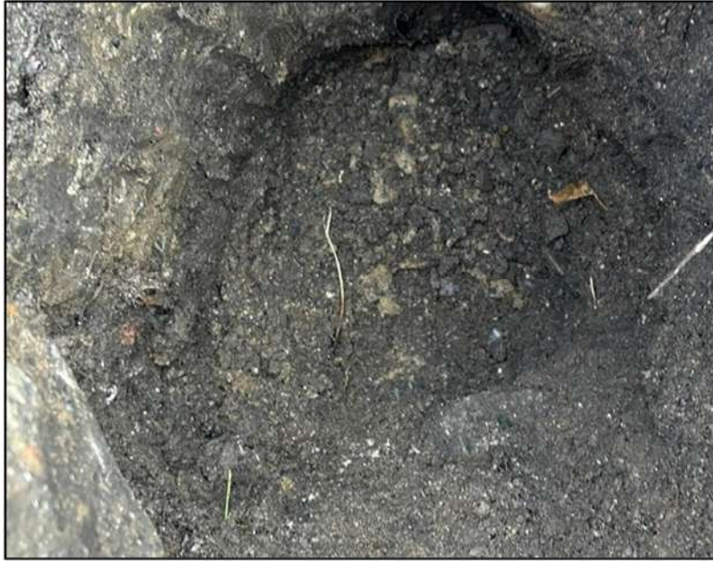
Insert 7 - Possible weathered bedrock encountered in HP201 and HP202. (Note: ground conditions within this stratum were too difficult to extract samples via hand excavation)
