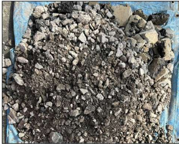
Insert 3 – Probable Sub-base encountered in HP202 to HP204 beneath the paving slabs
