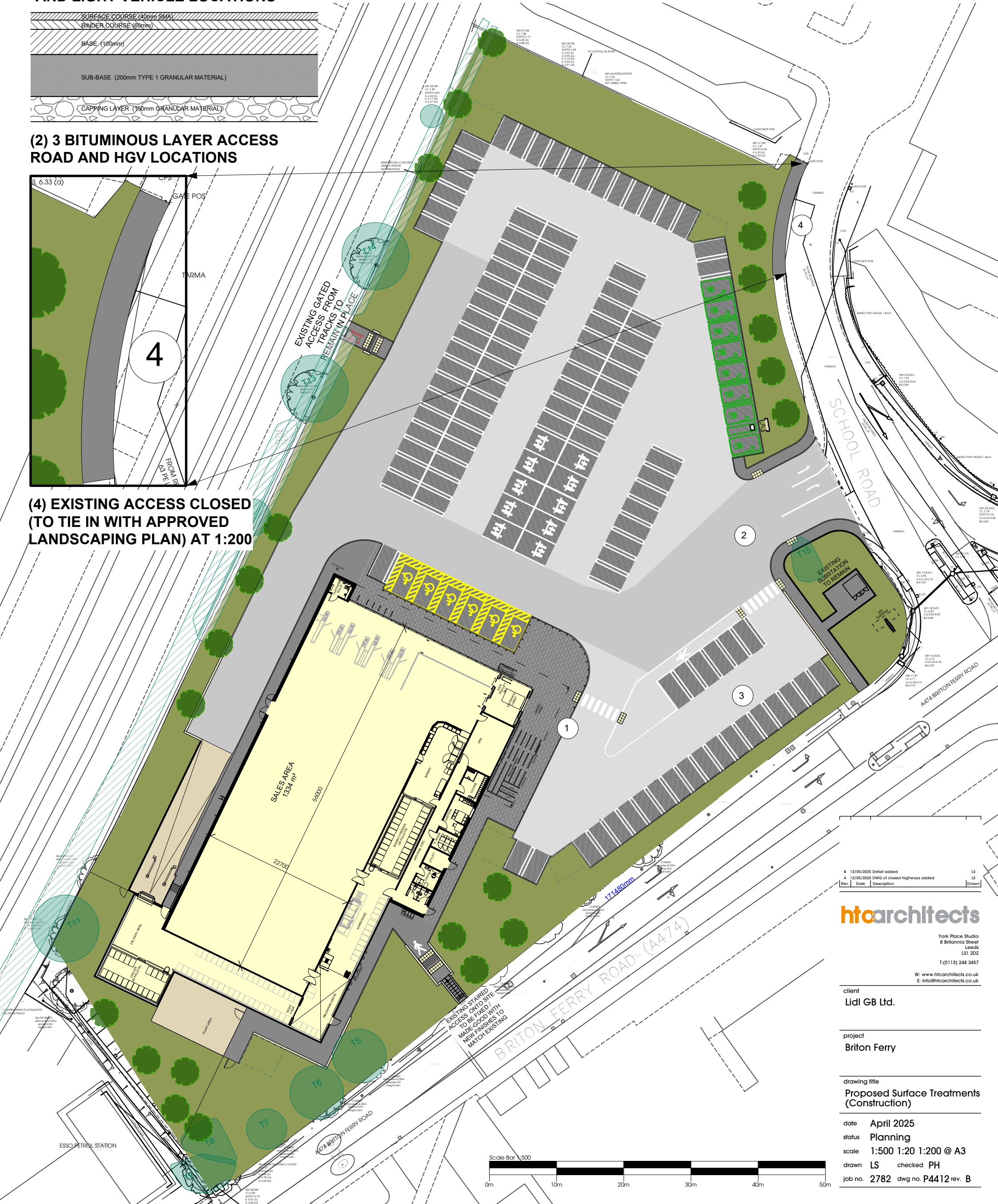
(1) 125MM WIDE FLAT TOP CHANNEL BLOCK ON 2 BITUMINOUS LAYER AND LIGHT VEHICLE LOCATIONS
