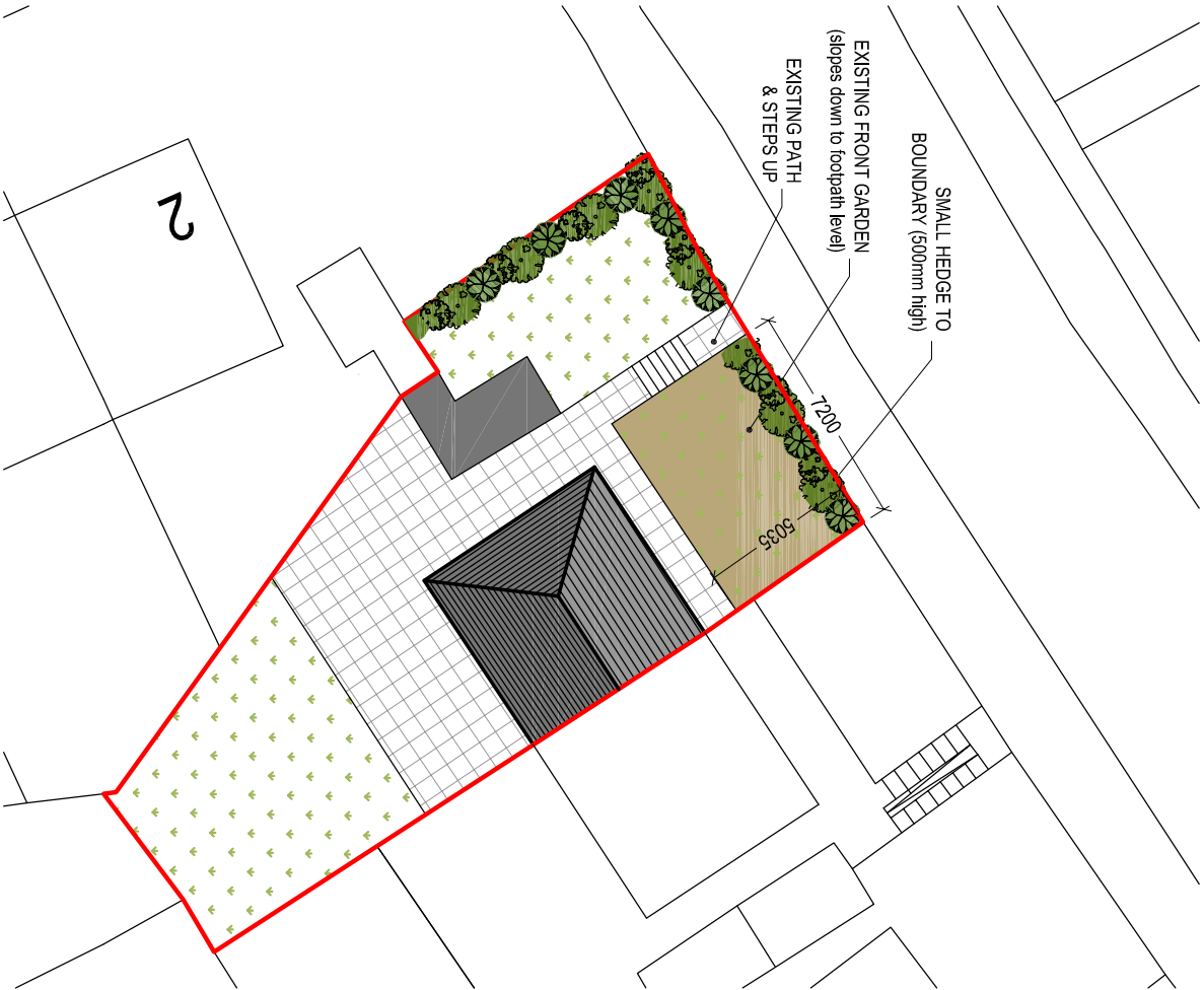
EXISTING SITE PLAN Scale 1:250
