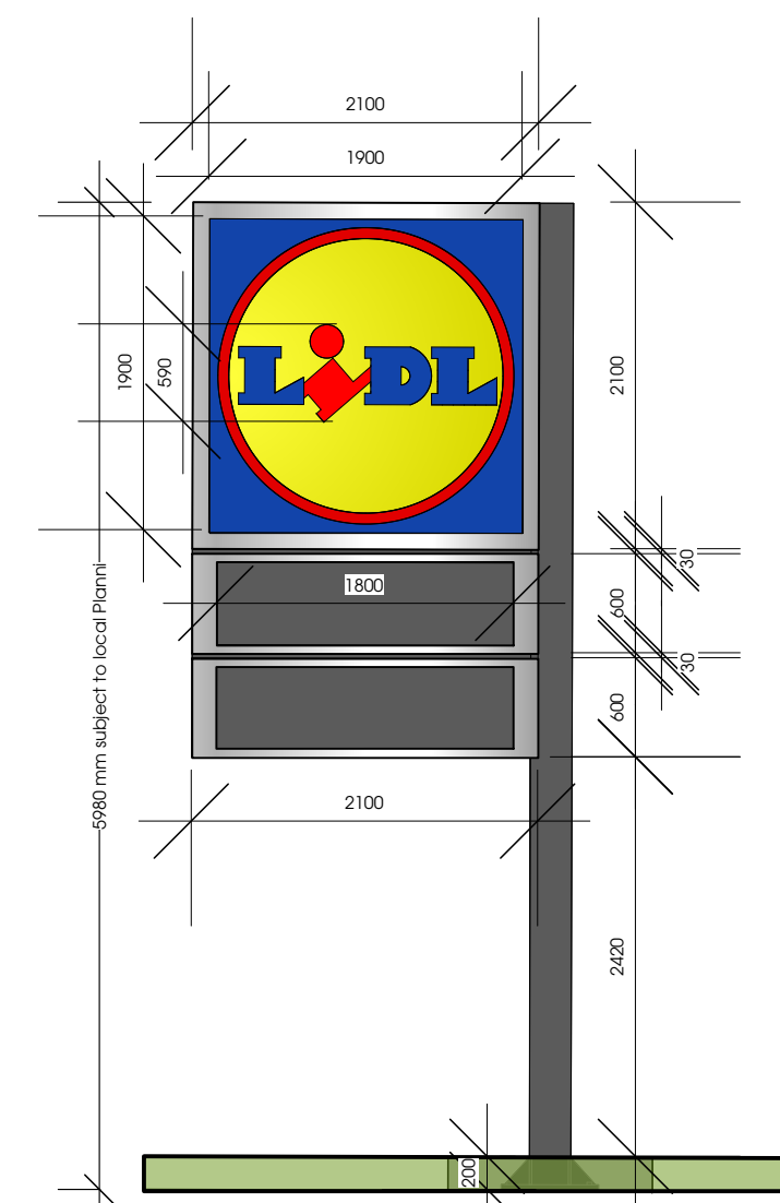
Flagpole Signage - Front Elevation
