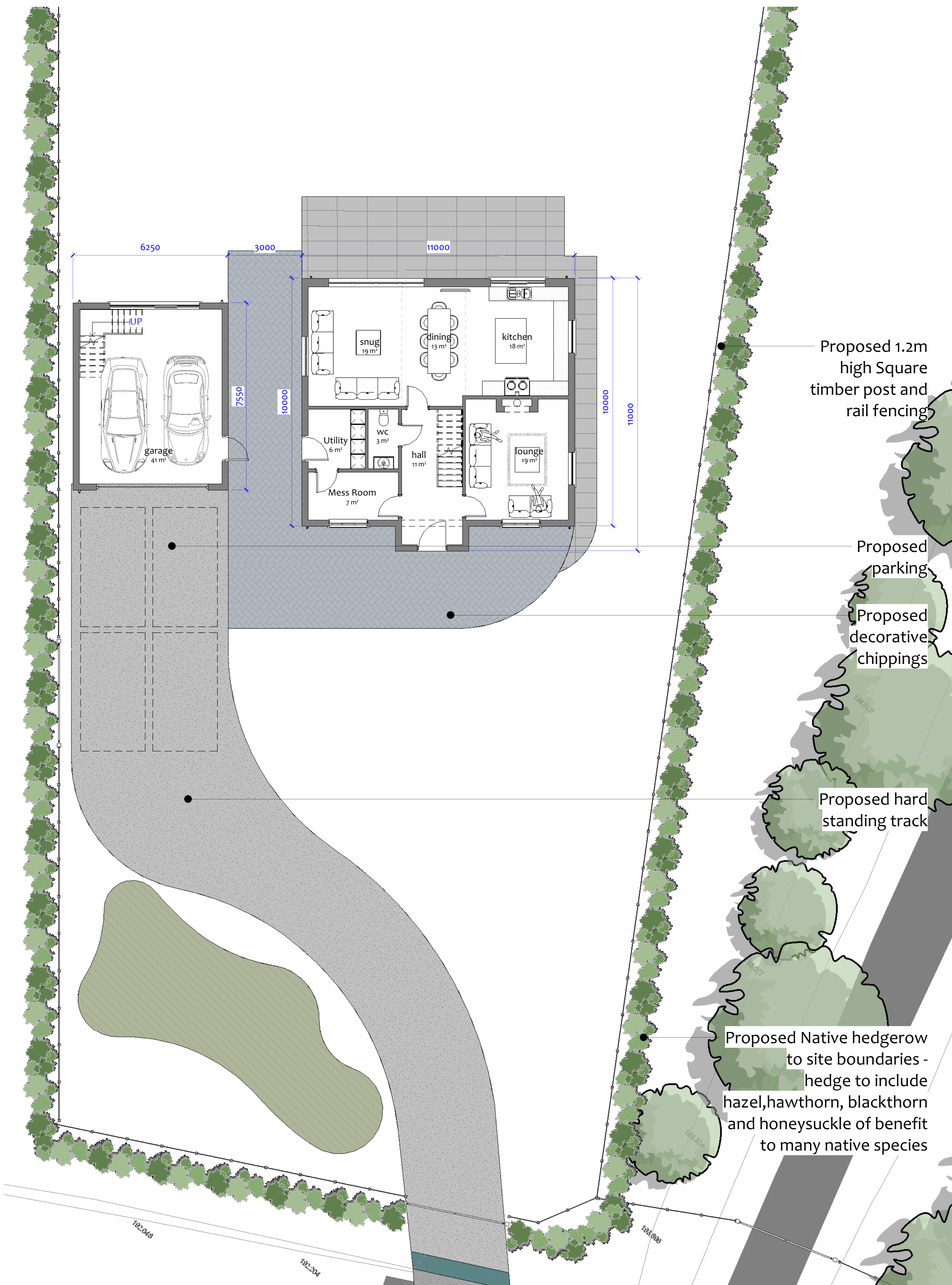
01 Ground Floor Plan 1 : 100
