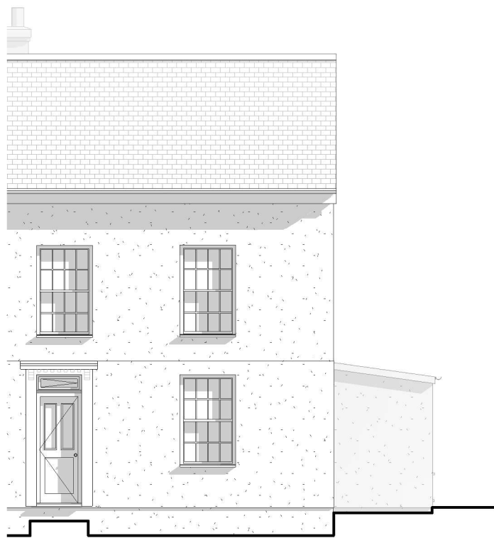
Existing North-West (Front) Elevation Scale 1:100 @A3
