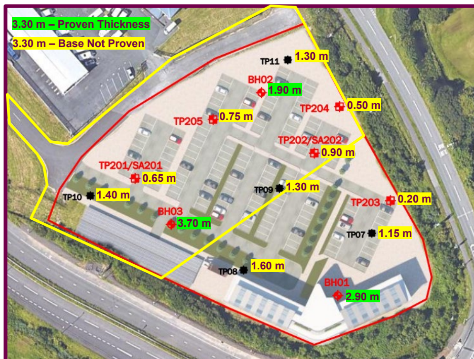
Figure 4 – Thickness of Blown Sands across the Application Site and immediate area
