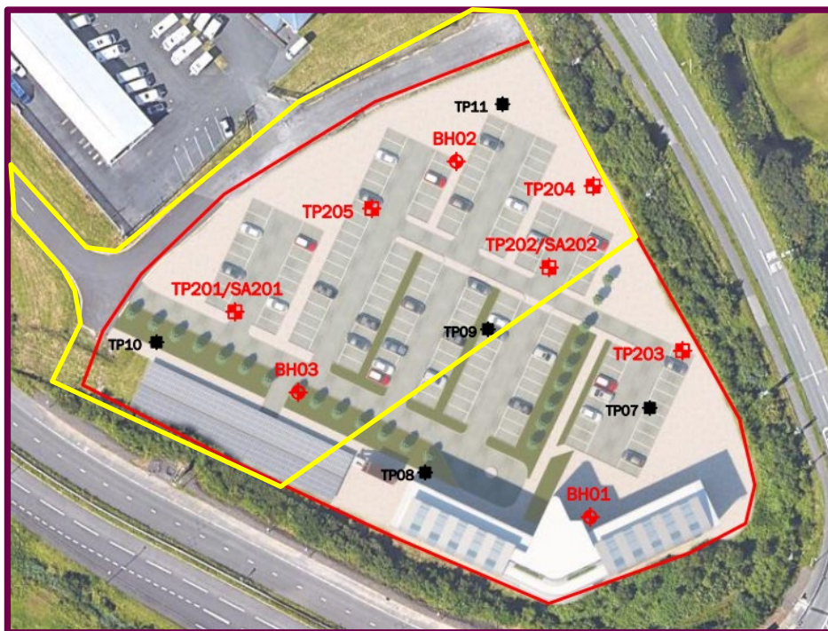
Figure 3 – ESP 2018 Area of Investigation and Exploratory Hole Location Plan
