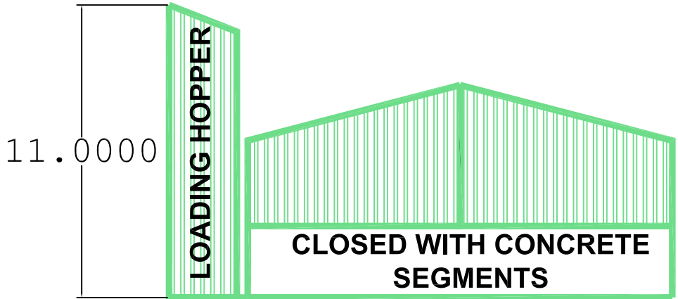
GABLE ELEVATION FACING SOUTH WEST( LOWER SECTION CLOSED WITH CONCRETE SEGMENTS)
