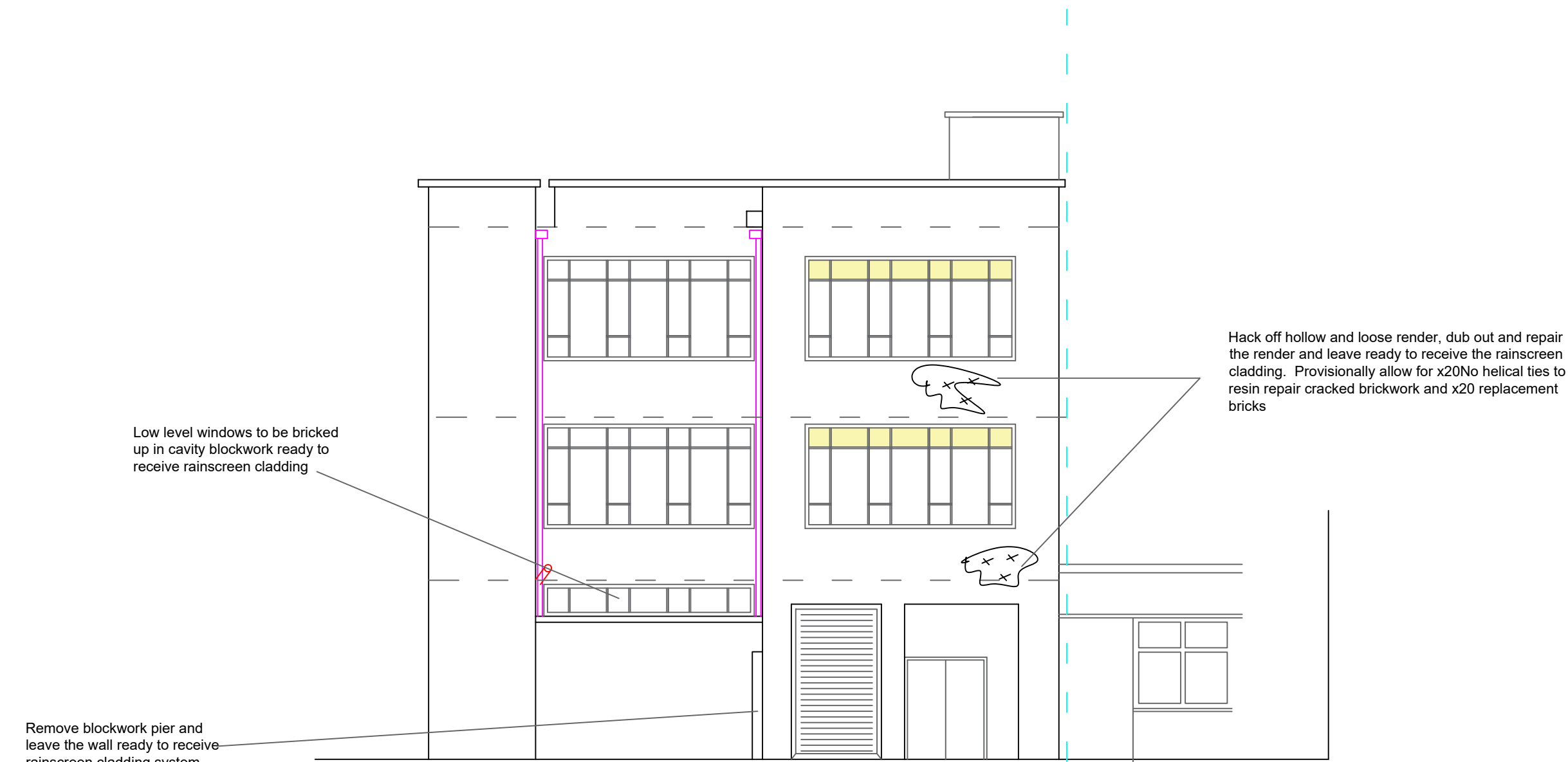
Existing Rear Elevation (Queen St Back Rd - southwest)
