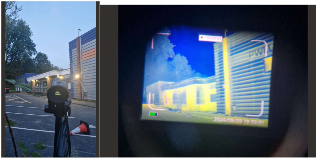
Figure 2 - Example of thermal camera position and view of structure
