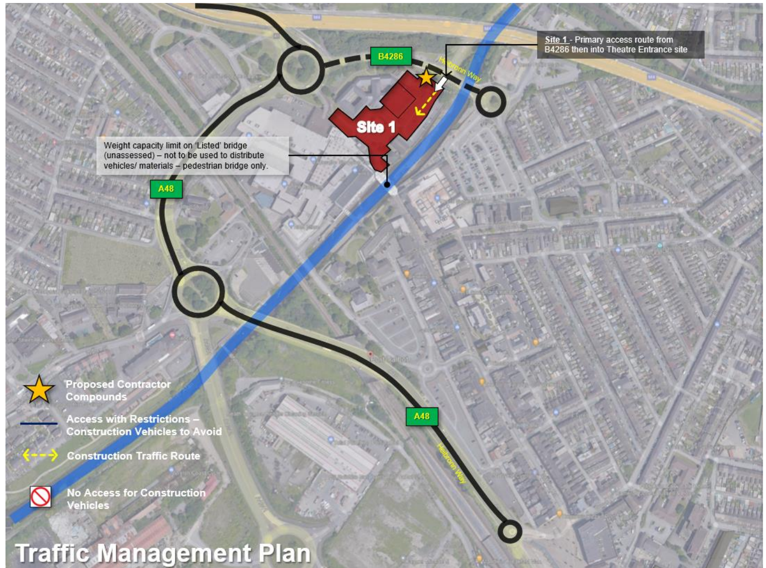
Construction access and egress to site 1
