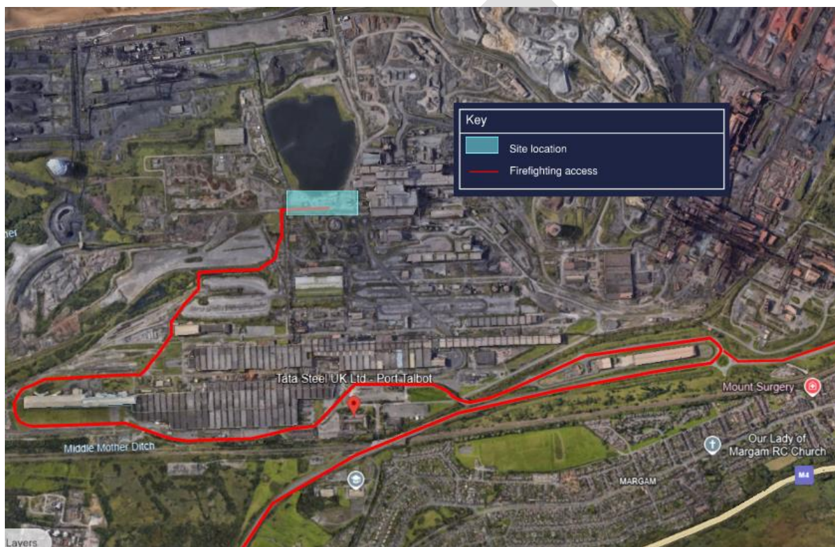
Figure 8: Firefighting Access (Source: Google Earth)
