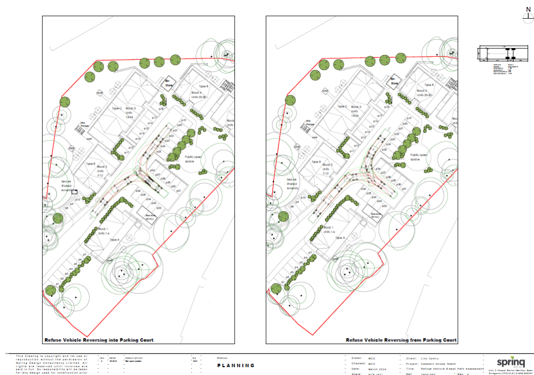
Figure 2.5 Internal Layout Swept-path Analysis
