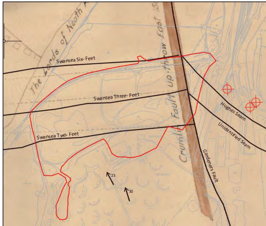
Figure 3: Excerpt from the abandoned mine recordings of various collieries (circa 1821) overlain with coal seam sub crops, geological faults and the Site boundary.
