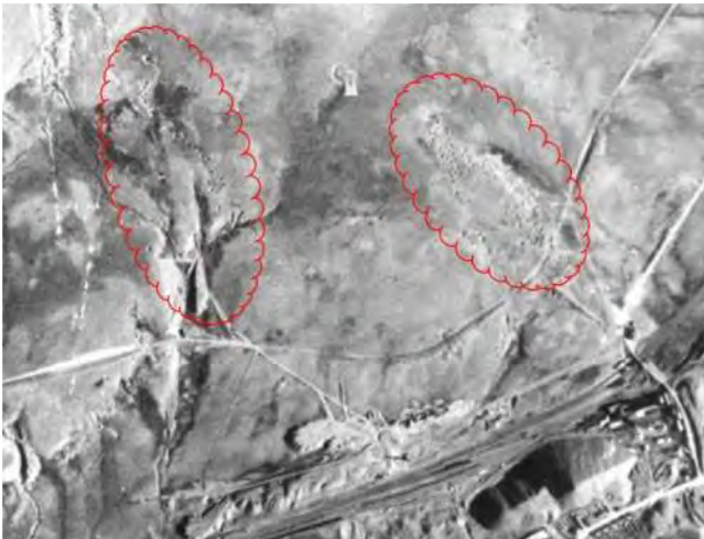
Figure 1: Extract from 1945 aerial photography showing potential “bell pitting”
