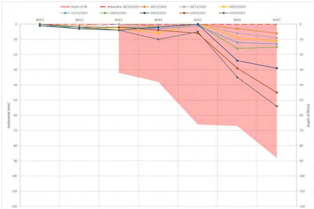
Figure D 4 Nant Helen Extension settlement monitoring results presented against depth of fill
