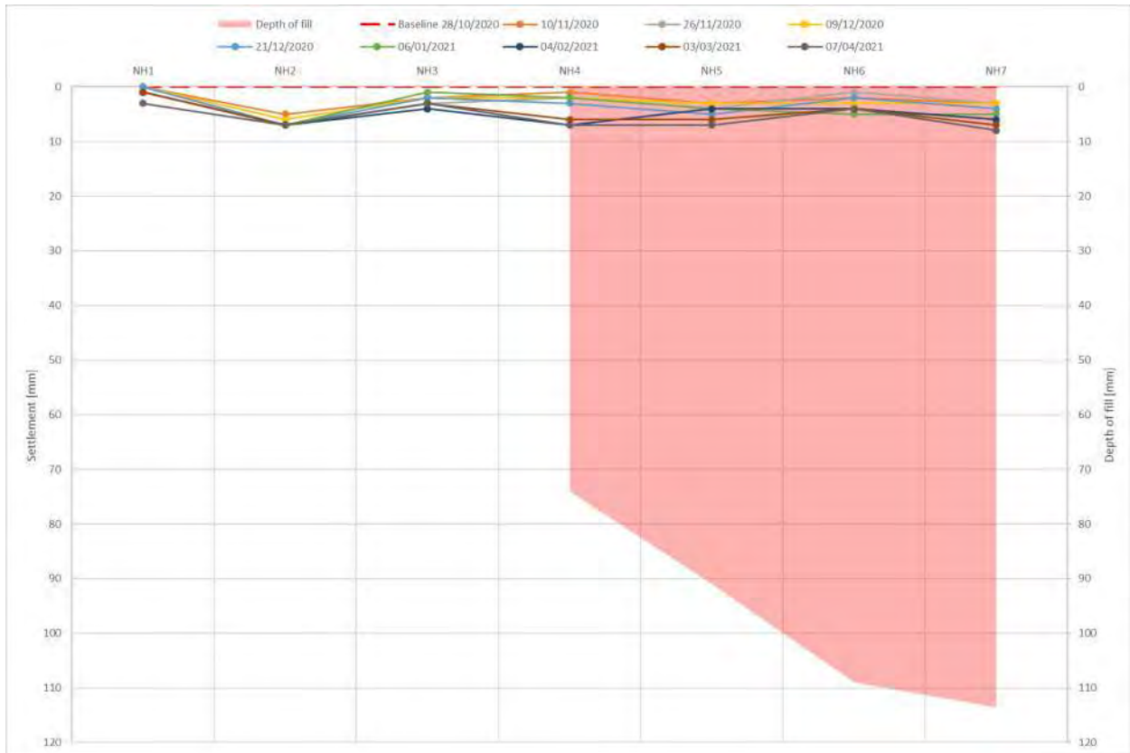
Figure D 3 Nant Helen settlement monitoring results presented against depth of fill
