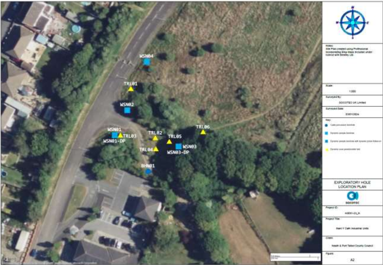
Figure 4.1 – Site Investigation Testing Location Plan
